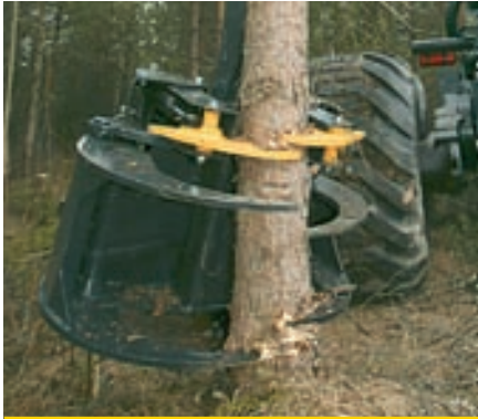
1. During the cutting stage, the grapple grips the tree and the guillotine cuts it.
