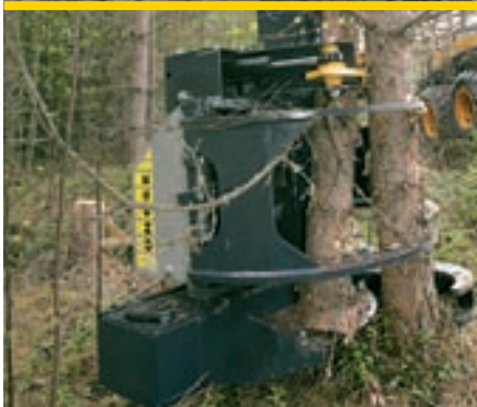
4. The operation continues until the grapple is full.
