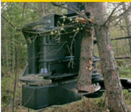
3. When felling more stems, the collection claws hold the cut stems in the grapple.
