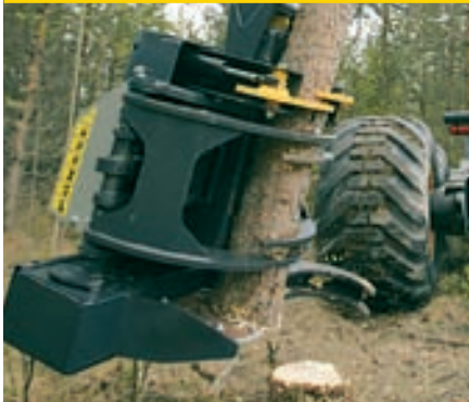
2. In conjunction with the cutting movement the stem passes automatically into the collection claws.
