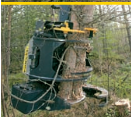
5. The guillotine blade acts as a guard preventing the cut stems from slipping downwards when working.
